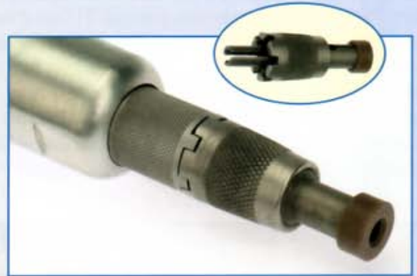
Nose assemblies are easily interchangeable
